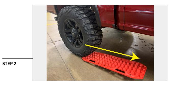
Drive onto the Recovery Boards to re-gain traction.
