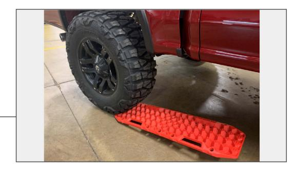
Place the Recovery Board under the vehicle's drive tires.
